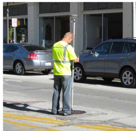
Survey Grade GPS Data Collection Used in the Collection of Sanitary Sewer System GIS
